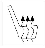
On vehicles with rear outboard heated seats, the buttons used to control this feature are located on the Rear Seat Audio (RSA) panel. (Heated Seat): To heat the seat cushion, press the button with the heated seat symbol.
